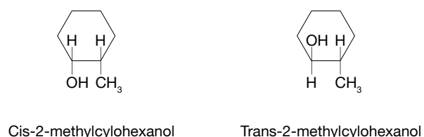
Figure 3.3 Cis- and trans-2-methylcyclohexanol.
