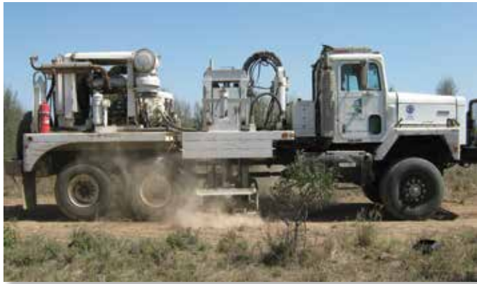
Figure 1.2 During a geophysical survey vehicles are used to create vibrations by hitting the ground. The vibrations are detected by sensors and the patterns produced used to create a view of the geology beneath.
