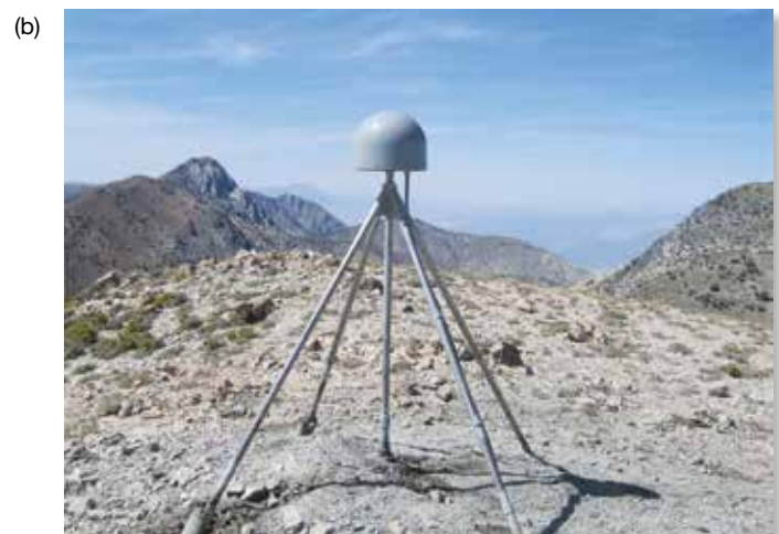
Figure 1.14 The movement of the Earth’s plates can be determined with the help of: (a) Satellite laser ranging (SLR) and (b) The global positioning system (GPS).
