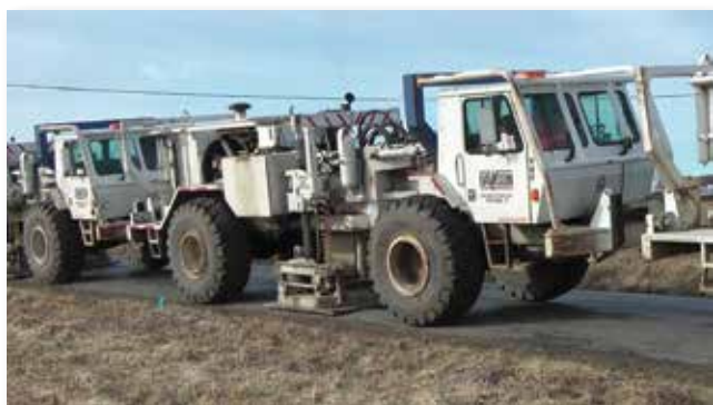
Figure 1.3 Geophysical survey These vehicles are used to create vibrations by hitting the ground. The vibrations are detected by sensors and the patterns produced used to create a view of the geology beneath.
