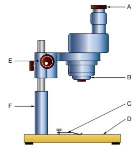
Figure 6.2 Side view of a stereo microscope.
