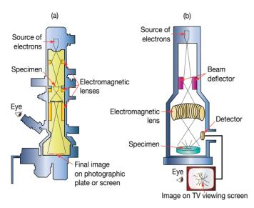
**Figure 7.2** Comparing electron microscopes. (a) Transmission electron microscope. (b) Scanning electron microscope.
