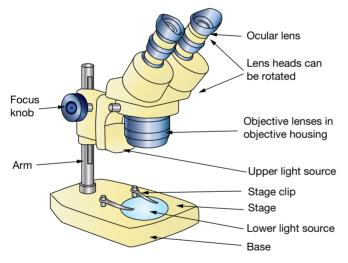
Figure 6.1 Stereo microscope.
