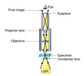
Figure 4.1 How light travels through a light microscope.
