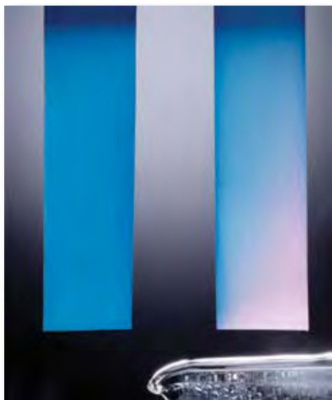
Figure 2.5 Cobalt chloride paper goes pink in the presence of water.
