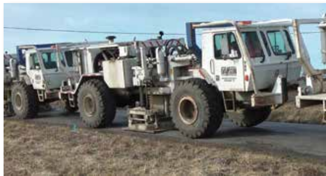
Figure 1.3 Geophysical survey These vehicles are used to create vibrations by hitting the ground. The vibrations are detected by sensors and the patterns produced used to create a view of the geology beneath.
