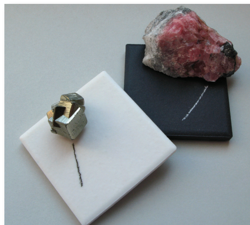
Figure 1.49 Streak plates Pyrite (left) and rhodochrosite (right) showing their characteristic streak colours.
