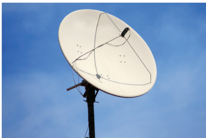
Satellite transmitter and receiving dishes use a concave reflecting system. The transmitter or receiver is at the focus of the concave dish.
