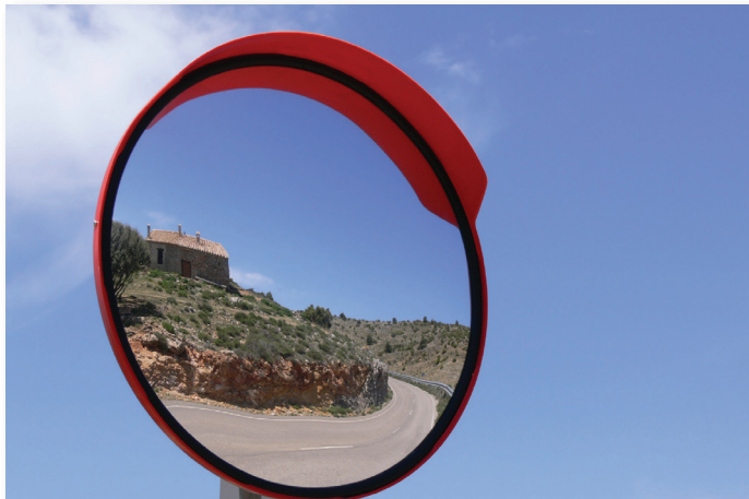
A convex reflecting surface can be used to see around tight corners on roads, or narrow driveways in building complexes.
