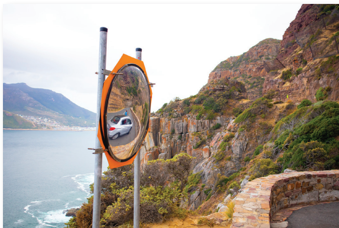
Convex reflecting surfaces can be used to increase the field of view of a traffic camera or a driver's rear view mirror.
